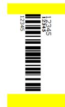
Here is an example of a label using ROTATION=1
